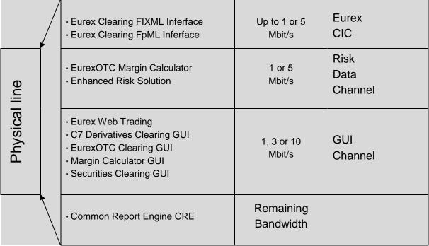
Figure 12: Configuration of CIC and additional channels
