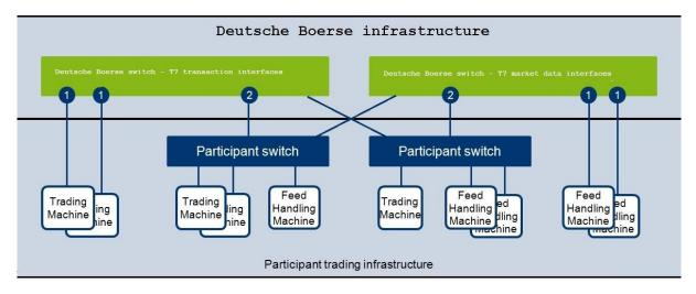
Figure 10: 10 Gbit/s peerless layer 2 connection to server or switch
